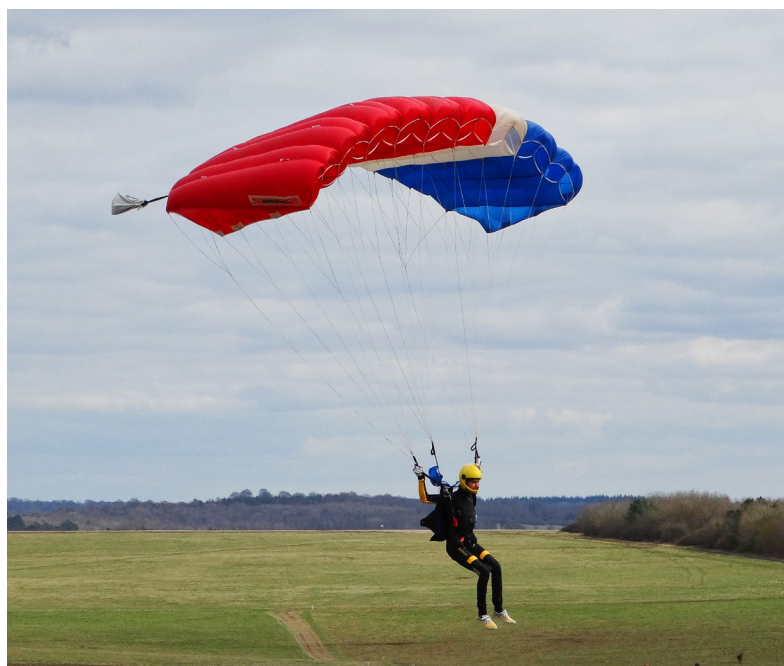
Figure 7: Using rear risers to extend the horizontal distance covered during the landing
