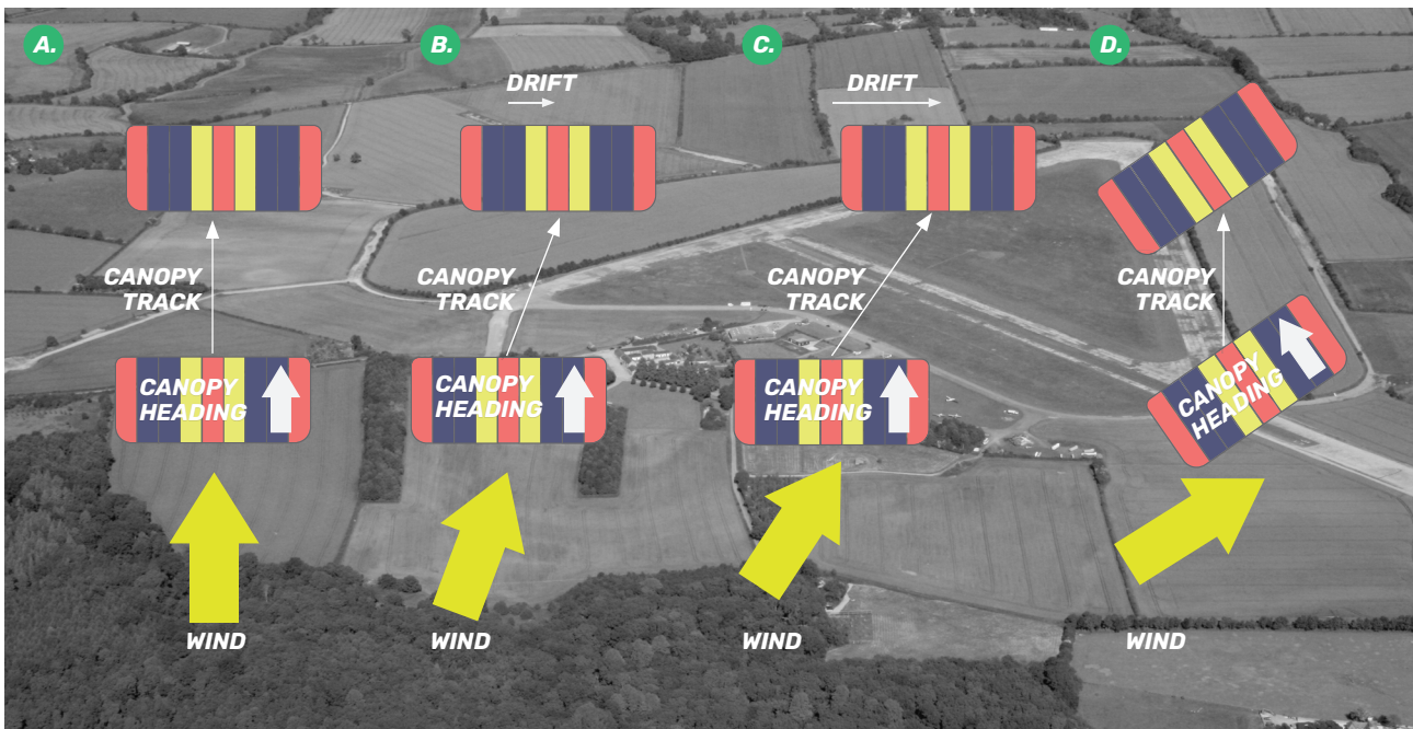
Figure 9: The difference between 'heading' and 'track'
