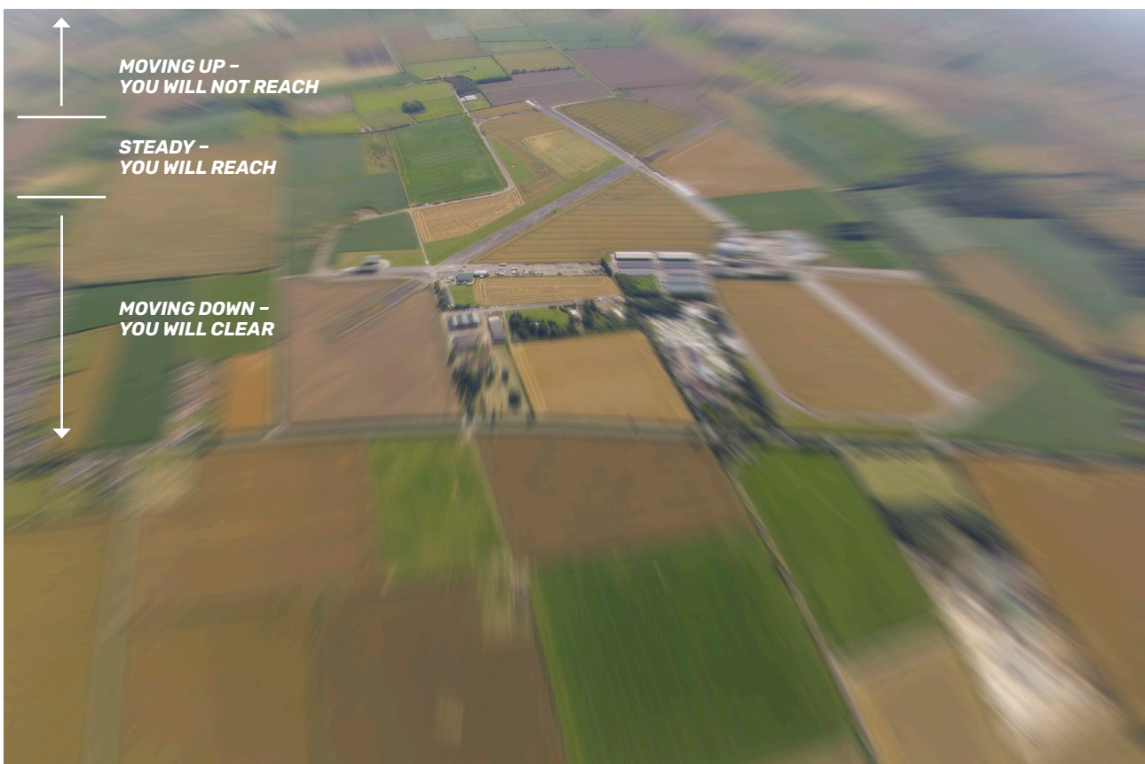
Figure 14: Finding the steady point with the accuracy trick
