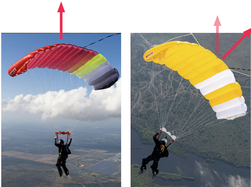
Figure 2: Lift in a turn (Photos Courtesy of Performance Designs)
